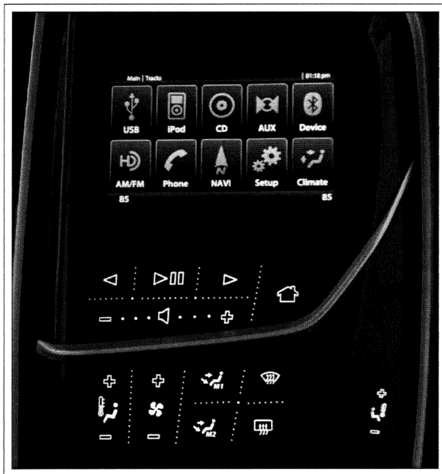
Fig. 3: A haptic touch screen shown by Visteon at the Consumer Electronics Show in January 2010 shows an automotive “infotainment” panel demonstrating the implementation of an 8-in. multifunction touch screen as part of an integrated control panel housed within the organic and flowing lines of a modern center-stack. Source: Visteon.
