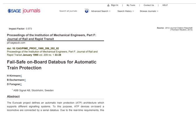
locomotive are connected by a serial databus. Due to the real-time requirements, this bus has to guarantee fast and deterministic response times. Due to safety requirements, this bus has to provide a high data integrity. Since the bus is not considered able to be trusted, safety applications have to implement a safe user layer on top of the usual bus protocols.
