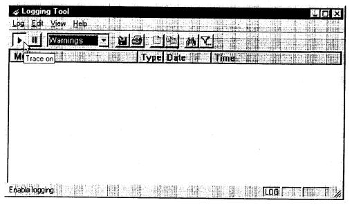
The log window will now record and display trace information as it is generated by Aventail Connect. You can tell when the trace function is active because messages are scrolling down the screen and the **Trace On** button is depressed.
