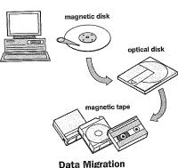
A data migration path in an HSM system might be from high-speed hard disk to slower speed optical disk to offline tape. In time, optical disks will almost surely replace magnetic media, but there will still be a need to take data off premises for protection against fire and accidents.
