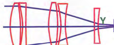
Lens With Field Flattener (Petzval Lens)
