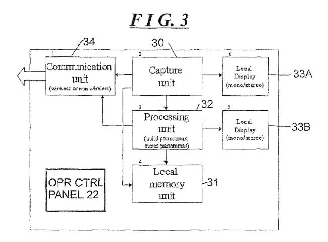
Figure 3 schematically depicts a functional block diagram of the stereoscopic data source according to the '284 Patent.
