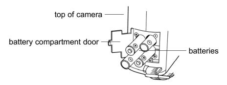
**IMPORTANT:** Make sure that you insert the batteries in the orientation shown in the above illustration.
