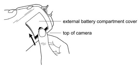
2. Remove the external battery compartment cover from the camera and set it aside.
