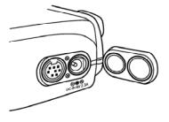
6. Plug the other end of the cable into the camera's serial port.
