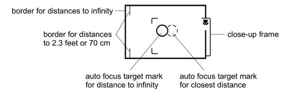
Consider the relationship of frames and focusing before you take a picture. The Auto Focus (AF) target marks are the solid and dotted circles in the viewfinder frame. The solid circle is the target mark for distance to infinity and the dotted circle is the target mark for the closest distance (up to 2.3 feet or 70 cm). If you are using the close-up focus mode, frame your subject within the small frame with the flower on the right side.
