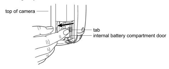
The door slides along its track and is released from its latch.
