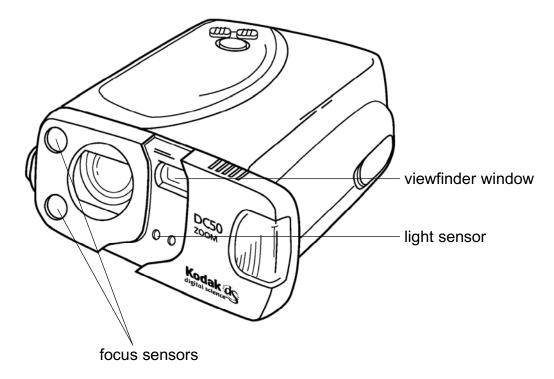
Clean the light sensors and focus sensors by rubbing them gently with a soft, dry cloth. Do not use any organic solvents to clean the sensors.
