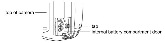
5. Pull gently on the tab in the direction of the arrow on the door.
