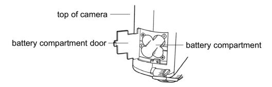
NOTE: The proper battery positions are indicated on the internal battery compartment door, as well as inside the battery compartment.
