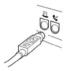
NOTE: If both ports are in use, disconnect the cable from one of the ports and connect the camera cable. Make sure that the cable is correctly oriented. Refer to your computer manuals for information about the ports on your computer.
