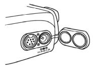
4. Plug the other end of the Macintosh cable into the camera's serial port.
