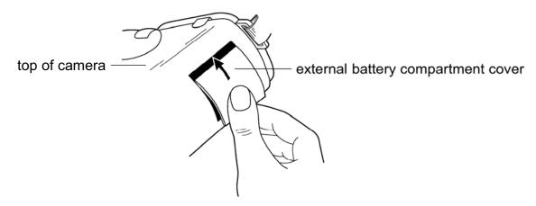
11. Slide the external battery compartment cover up until it locks into place.
