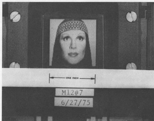
Fig. 11-18. Silicon Extrinsic Matrix: An array of transistors is fabricated on a single-crystal silicon wafer. The circuitry is similar to the TFT design with the liquid crystal in contact with the transistors. Silicon transistor action is much better understood and more reliable than TFT operation, but the substrate is opaque, expensive, and limited in area. An example of a picture displayed on a Hughes array is also shown. (John Gunther)
