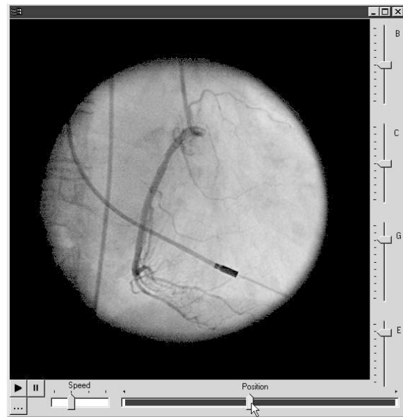
Figure 1. User interface for the DirectShow pipeline. The controls include play/pause (buttons in lower left-hand corner), playback speed, sequence position, brightness (B), contrast (C), gamma correction (G), and edge enhancement (E).
