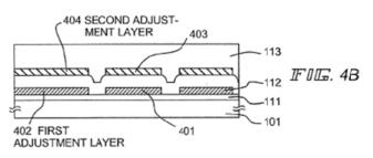
The adjustment layers 402 and 404 may be electrically isolated from the electrically connected auxiliary 401 and external connection 403 lines. (*Id.* at col. 4, 11. 45-48.)
