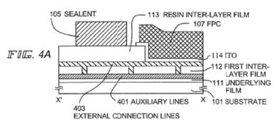
Figure 4A depicts external connection 403 and auxiliary 401 lines electrically connected together. As the figure shows, the lines extend under sealant 105. Figure 4A also depicts the flexible printed circuit 107 (FPC) electrically connected to an indium tin oxide (ITO) transparent conductive film 114 which is
