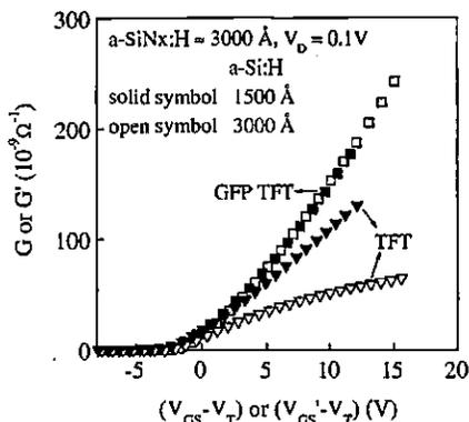
FIG. 1. Sheet conductance vs effective gate voltage characteristics for conventional *a*-Si:H TFT and GFP *a*-Si:H TFT structures having two different *a*-Si:H layer thicknesses. (*WL*) for the conventional *a*-Si:H TFT and GFP *a*-Si:H TFT are (56/16) and (100/20), respectively.  $V_T$  (1500 Å)  $\approx$  5.8 V and  $V_T$  (3000 Å)  $\approx$  2.5 V. Thickness of gate insulator (*a*-SiN<sub>x</sub>:H) is fixed at 3000 Å.
