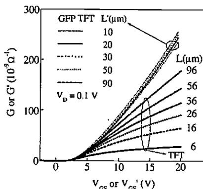
FIG. 2. Sheet conductance vs effective gate voltage characteristics for conventional *a*-Si:H TFT and GFP *a*-Si:H TFT structures having different channel lengths. *a*-Si:H and *a*-SiN<sub>x</sub>:H films are both about 3000 Å thick.
