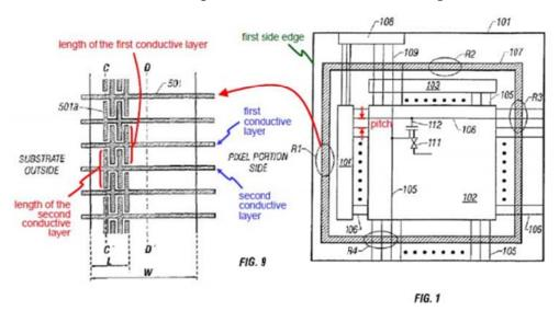
Figure 1 *supra* represents the top view of the lower substrate of an exemplary LCD device which incorporates, into the area R1 under seal 107, the dummy wiring structures depicted in adjacent Figure 9. (*See* Prelim. Resp. 14-16.)
