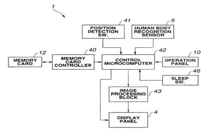
As shown in Figure 6 of the '828 patent, image display apparatus 1 has memory card 12, memory card controller 40, control microcomputer 42, image processing block 43, and display panel 4 (e.g., a liquid crystal display (LCD)). *Id.* at 3:38-41; 5:48-59. To display an image recorded in memory card 12, control microcomputer 42 reads the compressed image data from
