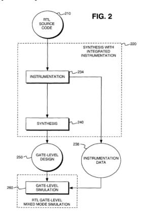
Figure 2, above, shows that RTL source code 210 is provided to synthesis process 220, which includes instrumentation step 234 followed by synthesis step 240. *Id.* at ll. 11-16. In the first embodiment, in which the gate level netlist is modified to include instrumentation signals, the resulting gate-level design 250 "contains additional logic to create the additional instrumentation output signals referenced in instrumentation data 238." *Id.* at ll. 17-30.
