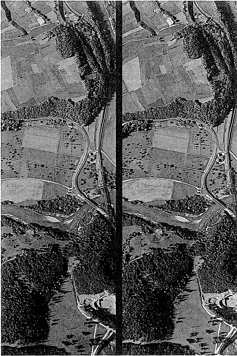
Color stereopair of Bonaduz, Canton of Grisons, Switzerland, October, 1975, photographs taken with Wild Leitz aerial camera RC10. Scale about 1:11,000.
