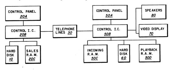
Figure 1 of the '573 patent is reproduced below:
