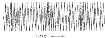
Figure 4. A frequency modulated radio signal, modulated by the same audio signal as in Fig. 3.
