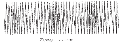
Figure 4. A frequency modulated radio signal, modulated by the same audio signal as in Fig. 3.
