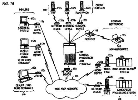
\*1318 '841 Patent, fig. 1A. An important feature of the invention was to allow the dealer to fill out a single application, to control which banks would receive the application, and to control the order and timing in which the applications were sent to the banks.
