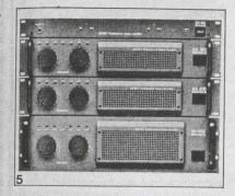
4. JBL AMP. The JBL 6215 Power Amplifier is a rack-mount unit designed for minimal power requirements such as monitoring through headphones or small speakers. The 6215 puts out 35 watts per channel into 8 ohms, 45 watts into 4 ohms, and 90 watts into 8 ohms in mono mode. JBL, 8500 Balboa Blvd., Northridge, CA 91329.
