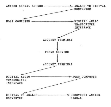
Fig. 1. System configuration diagram.
