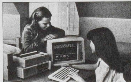
The IBM PCjr Enhanced Model includes a slim-line diskette drive, 62-key infrared keyboard and 131,072 characters of user memory.
