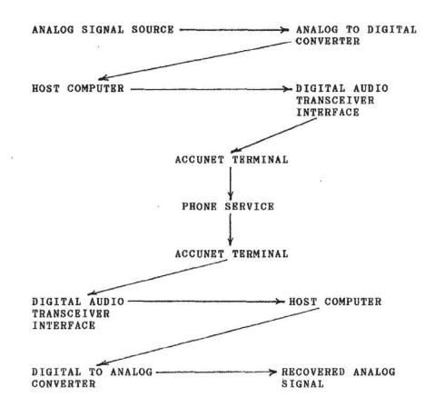
Fig. 1. System configuration diagram.
