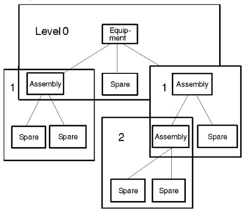
The BOM structure is reflected in the different technical types of BOM offered in the PM System:
