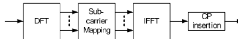
Figure 5.2.1-1: Transmitter scheme of SC-FDMA
