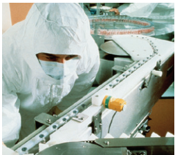
Manufacturing staffers oversee a filling machine to dispense final, formulated product into vials ready for distribution.
