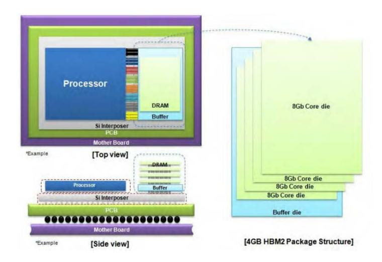
The 4GB HBM2 package is created by stacking a buffer die at the bottom and four 8-gigabit (Gb) core dies on top. These are then vertically interconnected by TSV holes and microbumps. A single 8Gb HBM2 die contains over 5,000 TSV holes, which is more than 36 times that of a 8Gb TSV DDR4 die, offering a dramatic improvement in data transmission performance compared to typical wire-bonding based packages.
