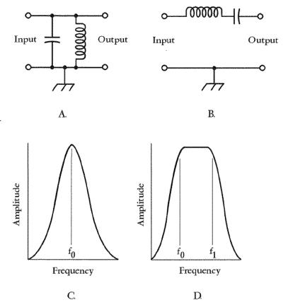
designed for the front end of a VHF or UHF radio receiver. A bandpass response is always characterized by high attenuation at all frequencies except within a particular range. The actual attenuation at desired frequencies is called the *insertion loss*.
