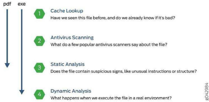
Figure 5: Example Sky ATP Pipeline Approach for Analyzing Malware
