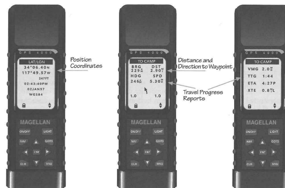
Figure 2-6: Examples Of The Three Basic Kinds Of Information Supplied By GPS Receivers
